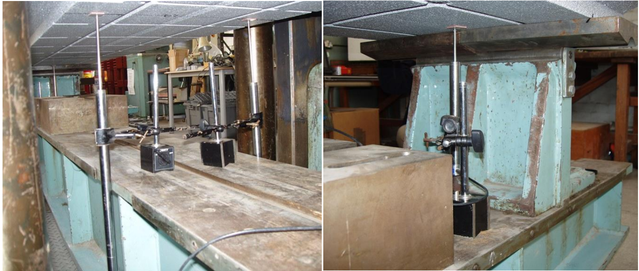
Figure 4. Displacement transducers at mid-span and close to the supports.
