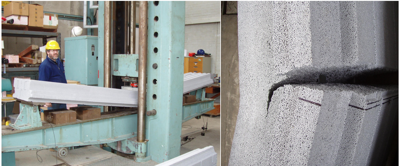
Figure 6. Tensile snap of the polystyrene at the bottom, across the mid-span (Test 1).
