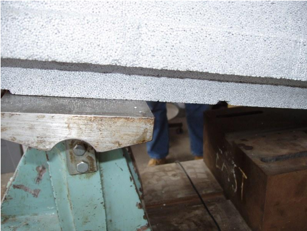
Figure 14. Compression in polystyrene at the supports was observed to be very small.
