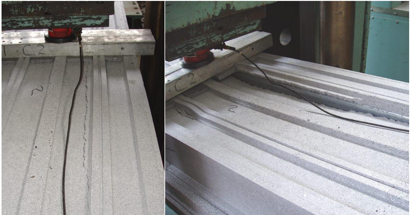
Figure 8. Tearing of polystyrene at the top surface spread along the panel and opened up exposing a steel 'C' profile with increasing deflection (Test 2).
