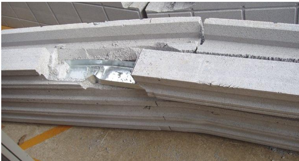
Figure 9. The exposed steel 'C' profile was observed to have bent about 400mm away from the mid-span (Test 2).
